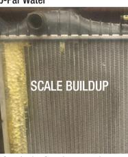
as efficiently. Only 1/16th of an inch of scale can reduce the cooling system heat transfer efficiency by 40%! This can result in overheating of the engine and corrosion at the hot spots.
